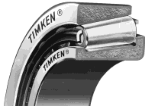
Fig. 1-7 Hardened case of bearing components provides fatigue resistance and the ductile core provides toughness.
