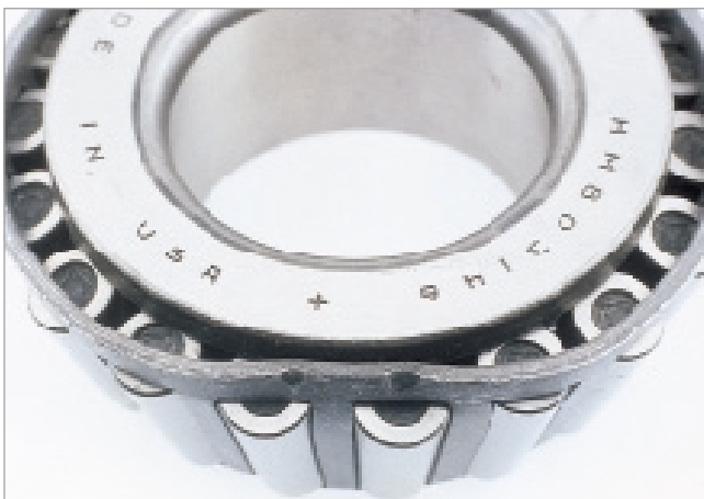
Cage deformation due to bad handling
