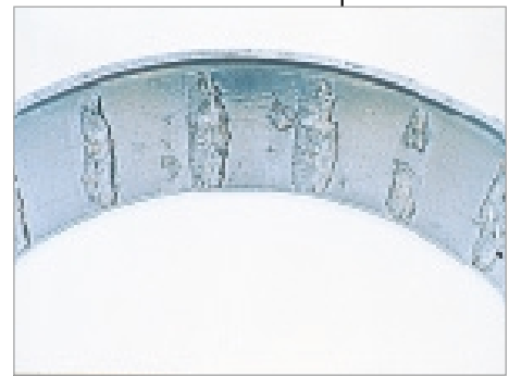
Spalling due to moisture etching
