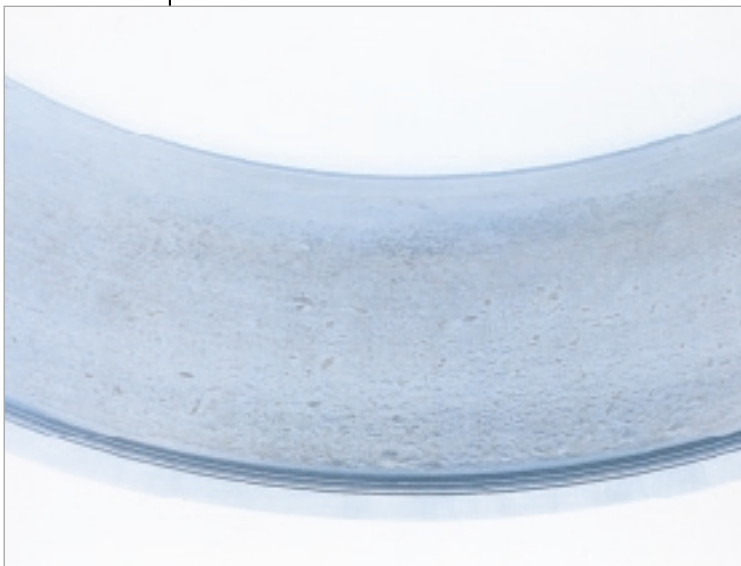
Fig. 4-17 Bearing damage due to particles
