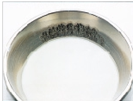
b) Geometric stress concentration on the cup due to misalignment
