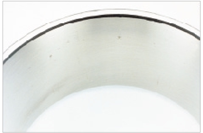
Nicks due to improper handling / mounting
