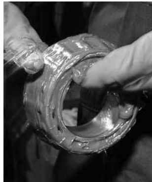
Fig. 23. Grease can easily be packed by hand.
