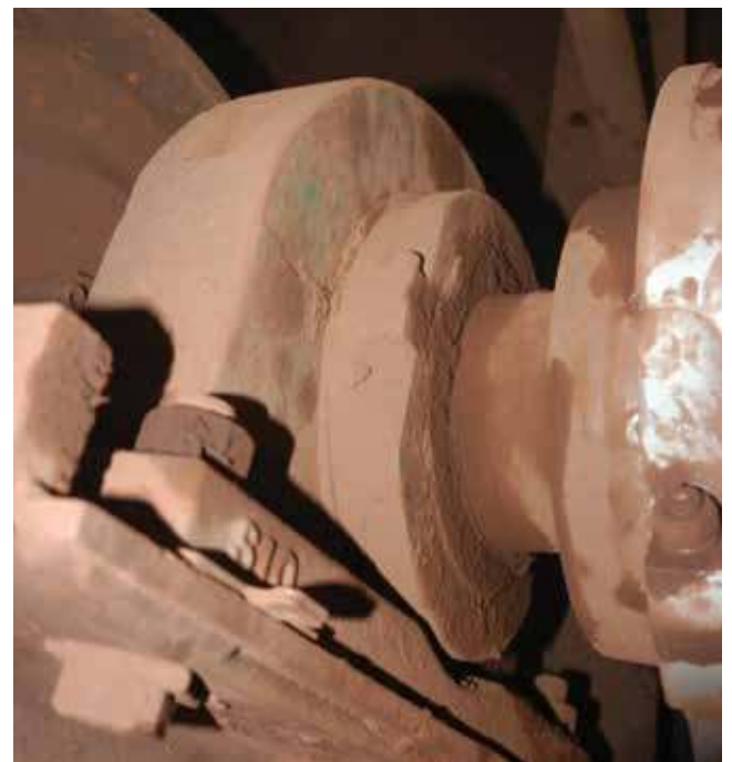
Fig. 20. Timken Split Cylindrical Roller Bearing Housed Unit is shown here in a steel industry application.
