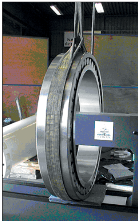
Induction Heating of a Large Bore Spherical Roller Bearing
