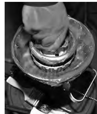
Fig. D-11. Mechanical grease packer.
