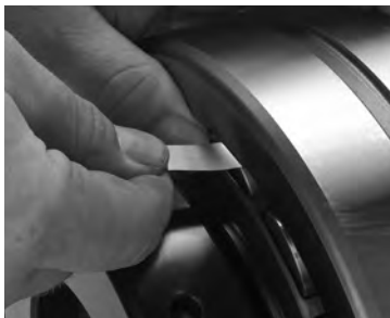
Fig. D-7. Measure RIC before installation.
