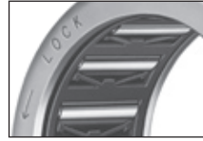
The mounted clutch and bearing assembly engages when the housing is rotated relative to the shaft in the direction of the arrow marking [← LOCK] stamped on the cup
