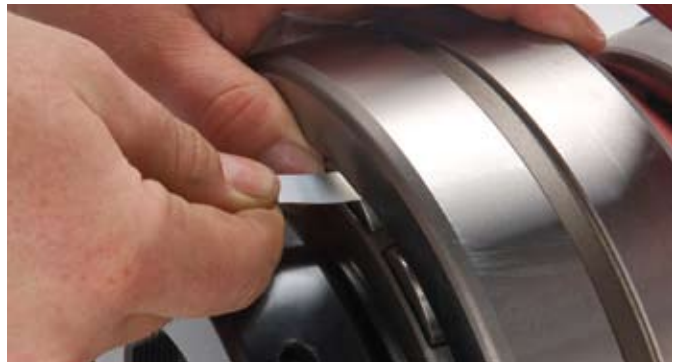
Fig. 30 Measure of RIC before installation
