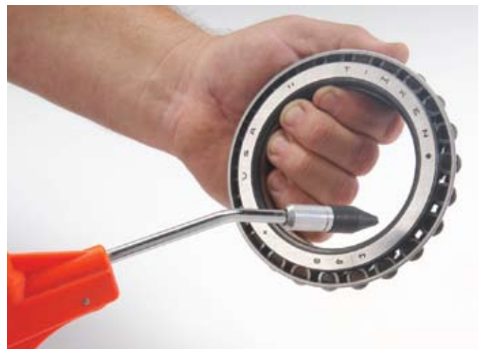
Fig. 19 Drying a bearing
