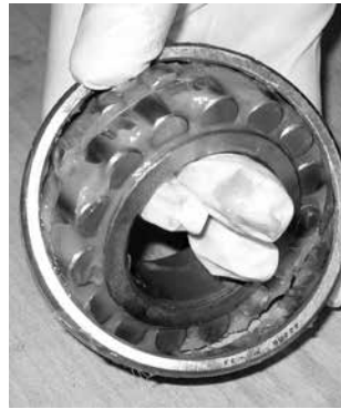
Fig. E-10. Grease can easily be packed by hand.
