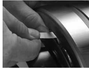
Fig. D-3. Measure RIC before installation.
