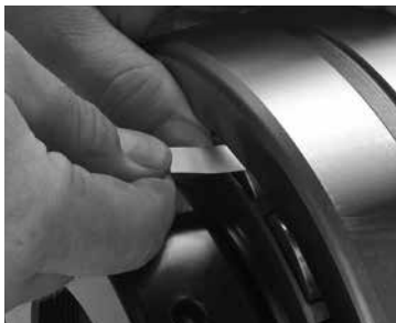
Fig. D-7. Measure RIC before installation.
