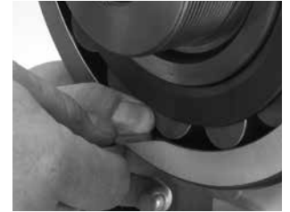
Fig. E-4. During mounting, the RIC should be checked at the unloaded roller.
