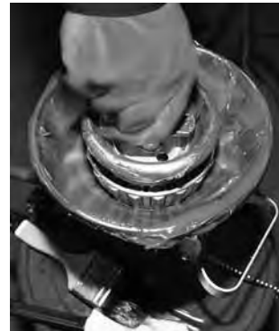
Fig. 15. Mechanical grease packer.
