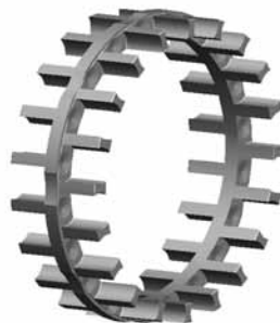
Fig. 4. One-piece finger-type cage.
