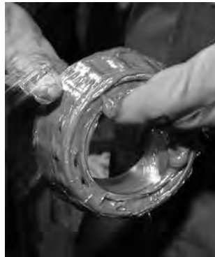
Fig. 14. Grease can easily be packed by hand.
