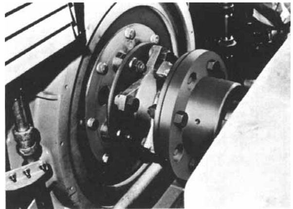
CMR coupling between engine and reciprocating compressor.
