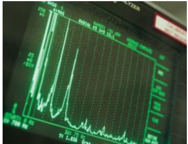
Functional testing — like this vibration analysis — is a critical and on-going part of Barden's quality control program.
