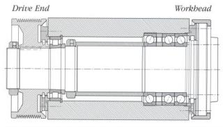
CNC spindle with a single row cylindrical roller bearing used in the drive end and a triplex set of angular contact ball bearings in the workbead end. This combination provides high speed and precision machining capabilities with high radial load carrying capacity.
