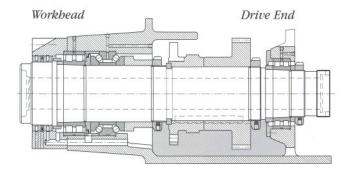
Heavy-duty latbe spindle showing a double direction angular contact thrust ball bearing used with a double row cylindrical roller bearing in the workbead. Drive end of the spindle features one double row cylindrical bearing. This combination allows spindle to operate with bigb rigidity, while accommodating both axial and radial loads.
