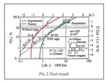
The reason for the increase of lifetime of linear bearings with caged technology is due to eliminating friction and reducing fatigue of the balls and the lubricant. The grease pockets in the caged ball form an active lubricant reservoir, which provides optimum lubrication during motion, and
