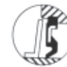
L TYPE SEAL. SBPP2( SET SCREW LOCKING ) SAPP2( WITH ECCENTRIC LOCKING COLLAR ),
