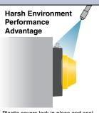
Plastic covers lock in place and seal against high pressure washdown Bearing stays free of liquids and particulates so inserts do not rust or fail prematurely.
