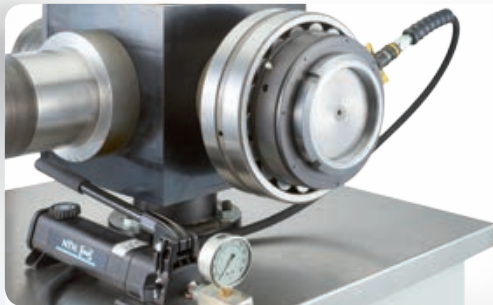
Extraction of the adapter sleeve with a hydraulic nut
