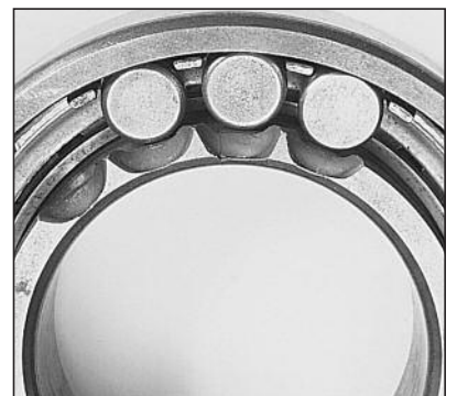
9 Nicks, cracks, fractures
