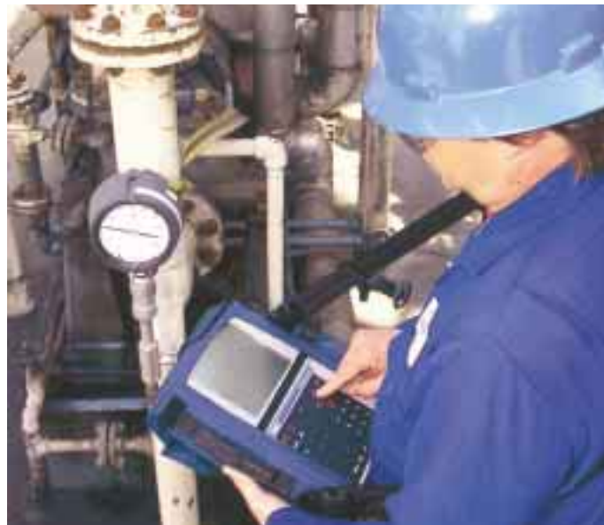
Microlog – portable data collector and analyser
