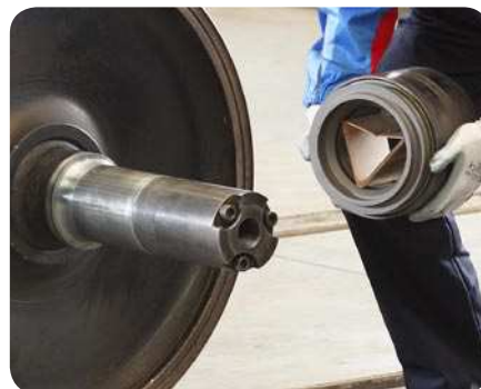
18 Preparing to install the tapered roller bearing unit including the backing ring
