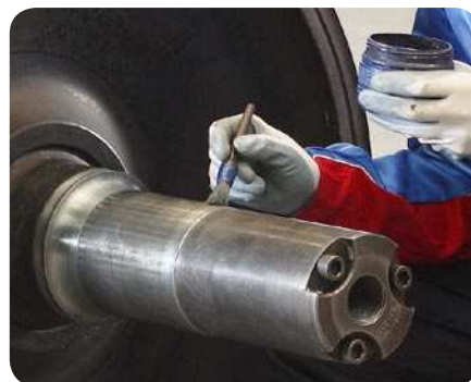
17 Coating the journal with a thin layer of light oil prior to mounting
