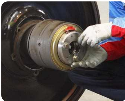
24 Installing the end cap
