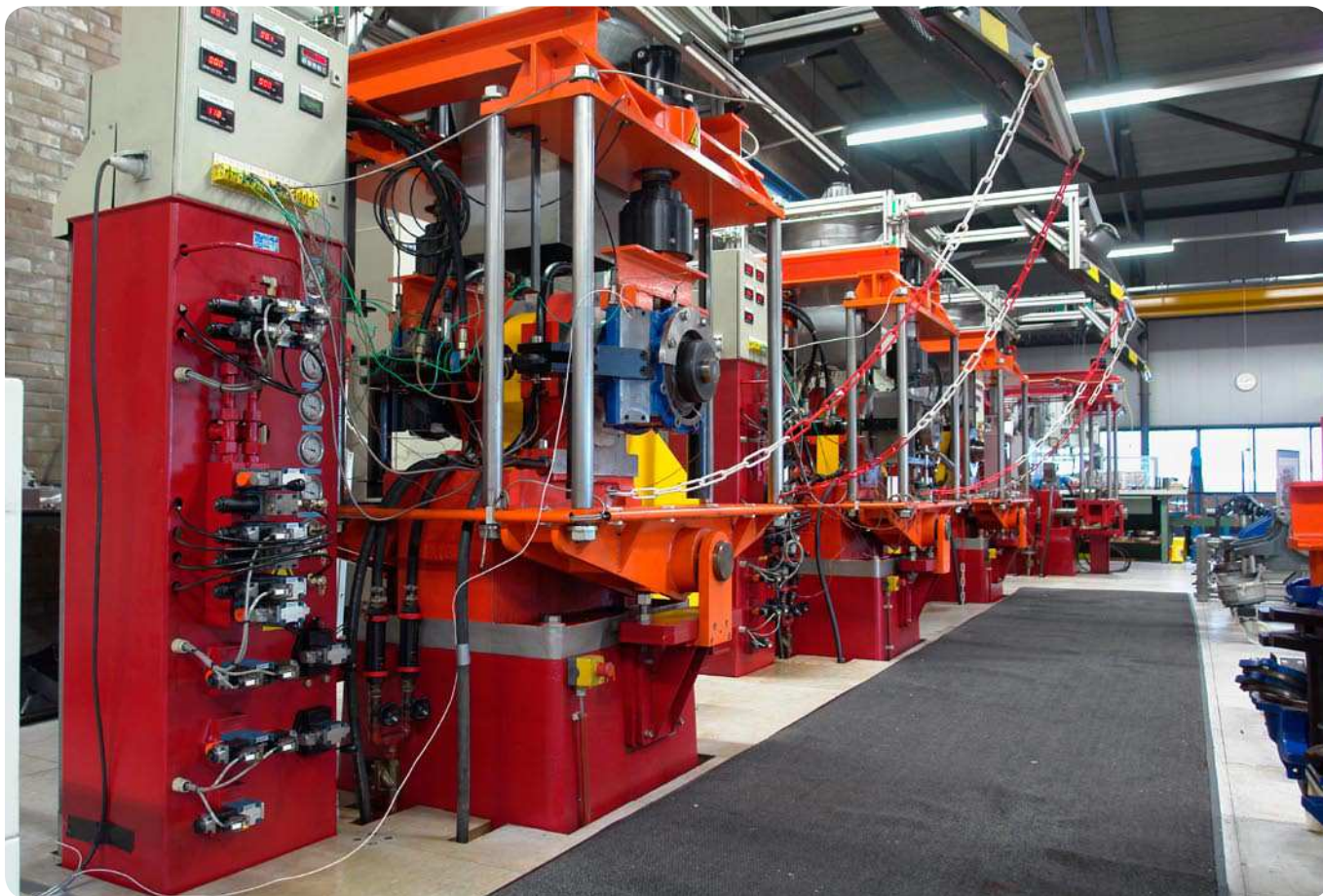
R3 endurance test rigs for quasi-static performance testing
