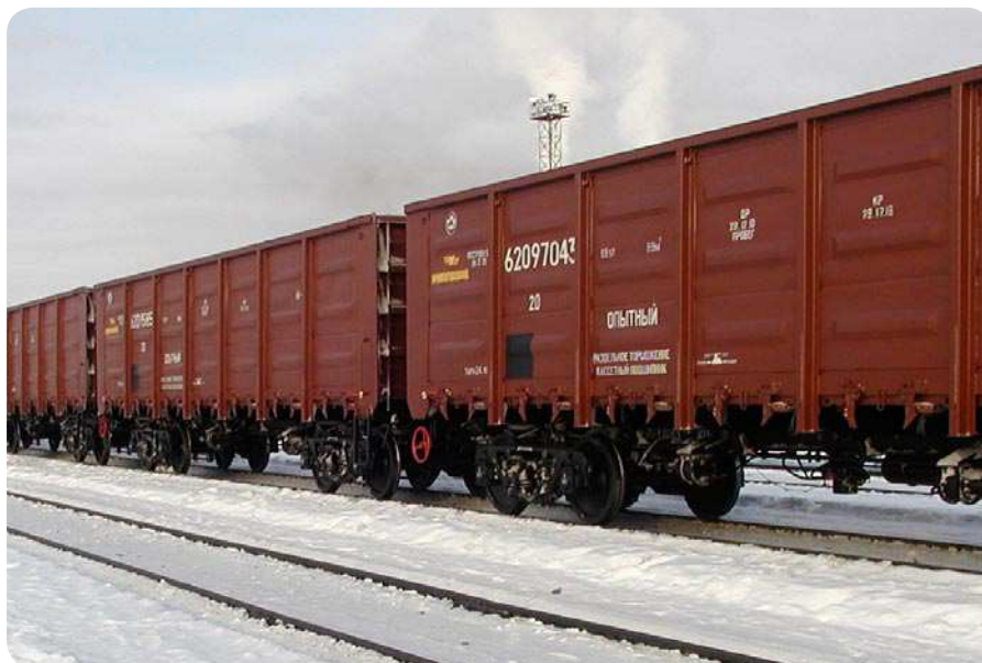
Field test with SKF axlebox bearing units Russian Vorkuta – Cherepovets coal railway line, 1 900 km long, max. speed 91 km/h, lowest temperature during the test –37 °C
