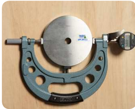
3 Calibrating the measuring device, using a master
