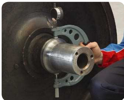
13 Checking the backing ring seat diameter, vertical position
