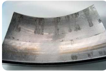
Rust marks on rolling element distance several sets due to stop and go
