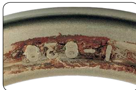
Without polymer spacer: strong fretting corrosion after 800 000 km
