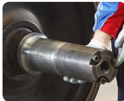
15 Attaching the pilot sleeve
