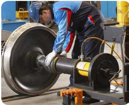
22 Pressing the TBU on its journal seat while rotating the outer ring by hand (→ page 185 )
