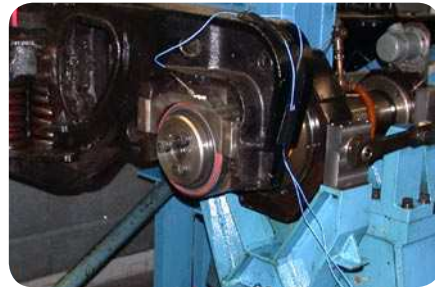
Left and right: THISBE test rig for high-speed bearings which can simulate dynamic load conditions equipped with an original bogie frame
