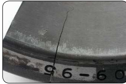
Cracked inner ring The bearing was fitted on an oversized journal.
