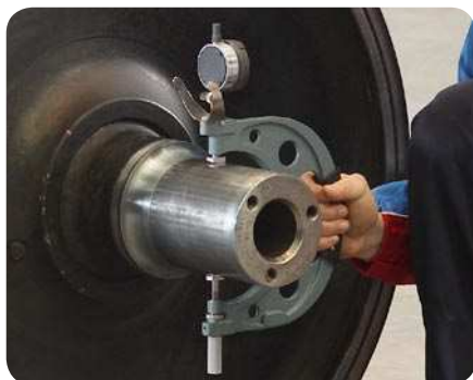
11 Checking the bearing seat diameter, journal inside, vertical position
