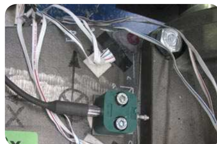
Application of strain gauges for stress level recording
