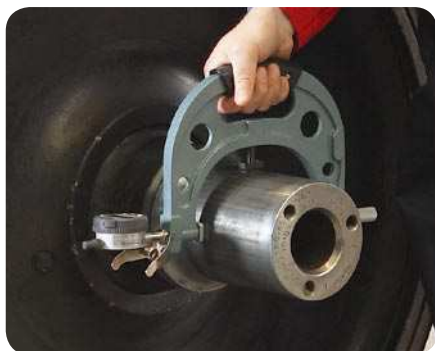
12 Checking the bearing seat diameter, journal inside, horizontal position
