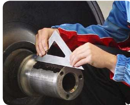
5 Checking journal straightness with a ruler
