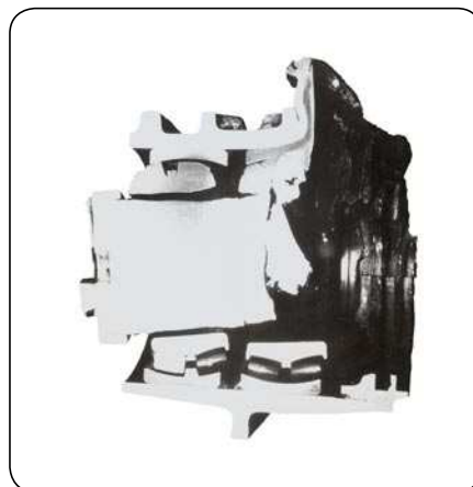
Axlebox after derailment (cut through)
