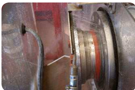
Watertightness test in operation
