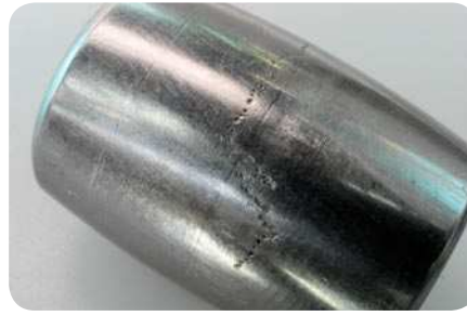
Heavy cratering on a spherical roller due to excessive voltage
