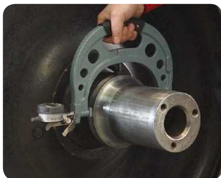
14 Checking the backing ring seat diameter, horizontal position
