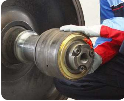
20 Sliding the tapered roller bearing unit to the end position on the pilot sleeve
