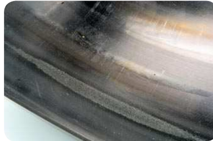
TBU outer ring with a large area full of craters The bearing should be scrapped.
