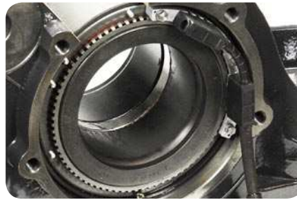
“Double head” SKF Axletronic speed sensor for automatic train control (ATC) and ETCS applications
