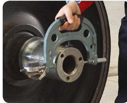
8 Checking the bearing seat diameter, journal end, horizontal position
