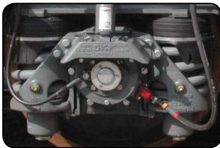
SKF Axletronic sensor applied in an axlebox front cover in combination with an earth return device Photo: Siemens
