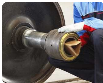
19 Installing the tapered roller bearing unit on the pilot sleeve
