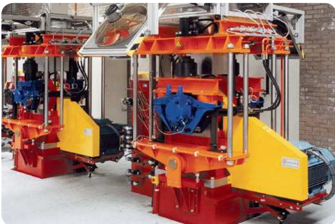
SKF R3 test rig arrangement in accordance with EN 12082
