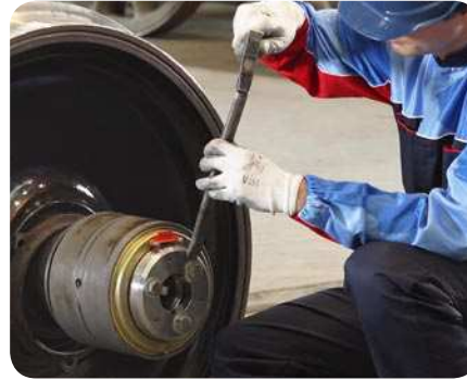
26 Bending the tabs of the locking plate
