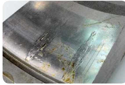
Impact during mounting or standstill Plastic deformation at roller distance. Spalling is starting.
