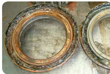
Fretting corrosion on a rear seal and rear inner ring. The grease is discoloured brown due to the fretting debris. The SKF polymer washer eliminates this problem and extends the service life of the grease and therefore the bearing.
