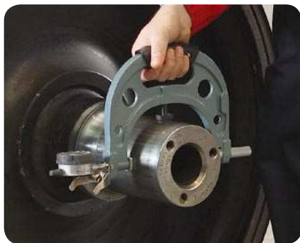
10 Checking the bearing seat diameter, journal middle, horizontal position
