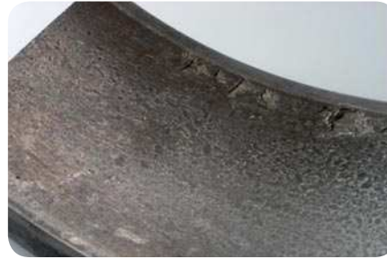
TBU outer ring with heavy indentation damage Spalling has started on one side of the raceway (top).
