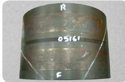
Fretting corrosion marks on the outer ring. The outer ring has a clearance fit in the housing. Note that the contact marks are not even or in line, suggesting an uneven load acting on the axlebox housing.
