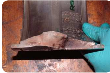
Due to heavy spalls and continuous loading, the material became fatigued and fractured all the way through.
