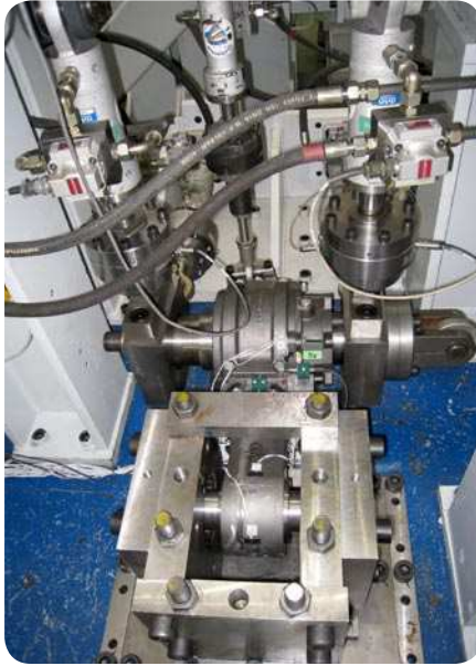
Fatigue testing of a high-speed axlebox housing
