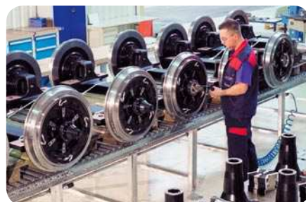
SKF axlebridge assembly line where components such as wheels, couplings, earth return and brake systems are mounted
