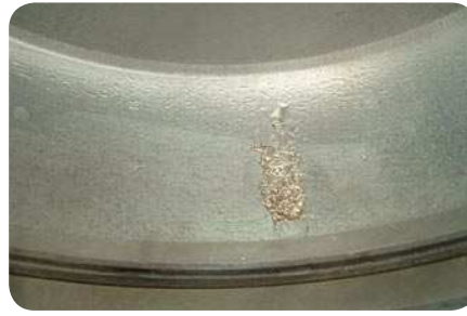
Sub-surface initiated fatigue in the outer ring load zone
