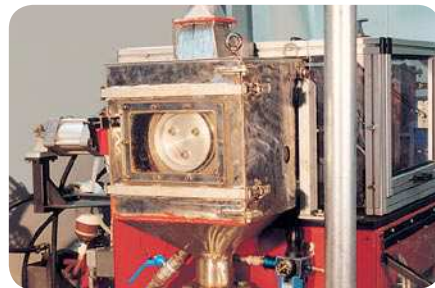
SKF environmental seal test rig for simulating contaminated conditions such as dust and water
