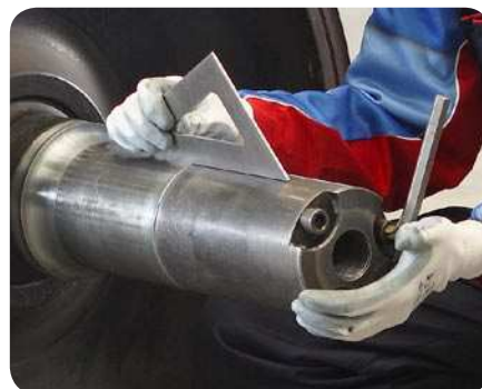
16 Checking the alignment of the mounted pilot sleeve in three positions: 0°, 120° and 270°
