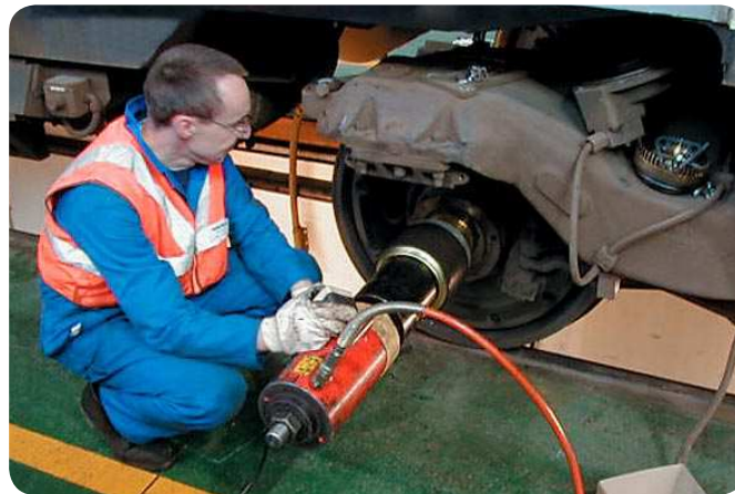
SKF service engineering offers special solutions such as bearing unit exchange without the need to dismantle the bogie or wheelset
