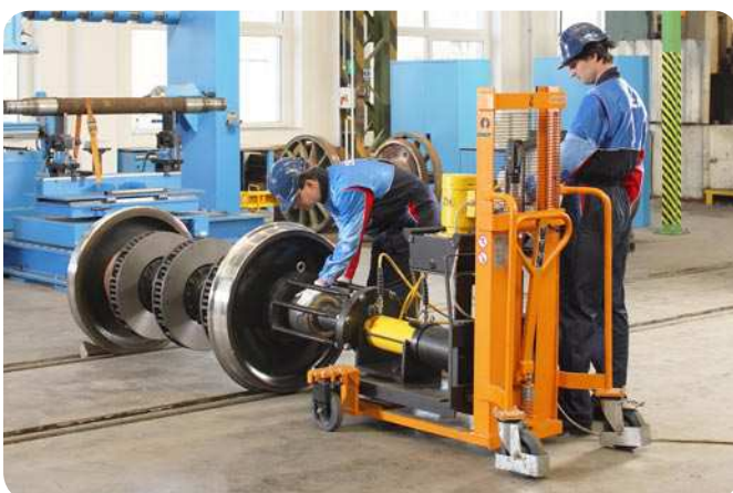
Adjusting the dismantling tool
