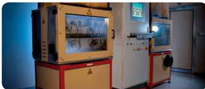
Idler endurance test rig
