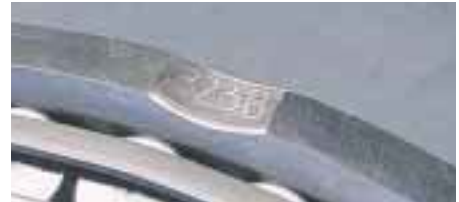
Marking of parts belonging together with serial number and letters
