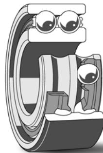
Double row angular contact ball bearing (data tables on page 69)
