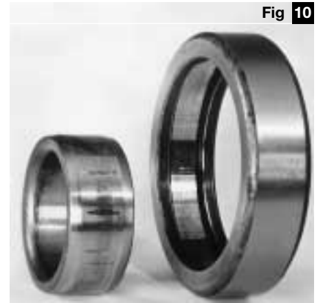
Inner and outer ring of a cylindrical roller bearing exposed to vibration The inner ring has changed position
