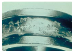
Stage 4: If run too long, the whole raceway is spalled; initial damage can no longer be observed.
