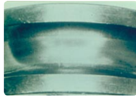
Stage 1: Fine roughening or waviness develops on the surface.
