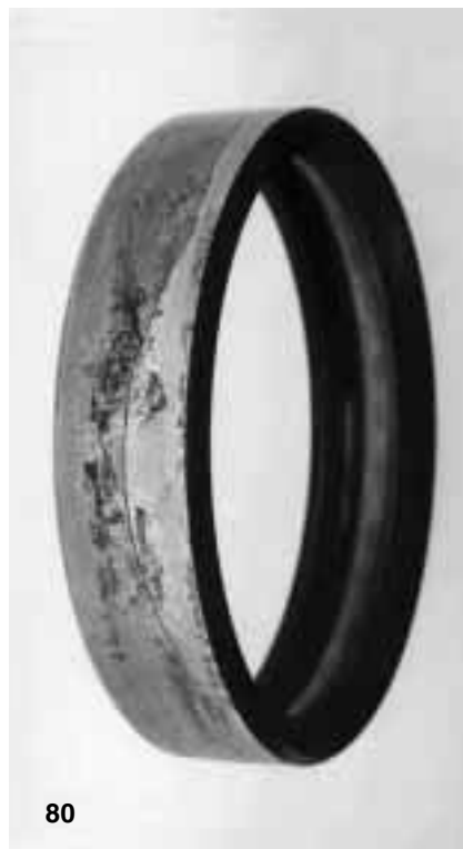
Fig 79 Spherical roller bearing inner ring with fretting corrosion and a transverse crack right through the ring. The fretting corrosion has caused the cracking
