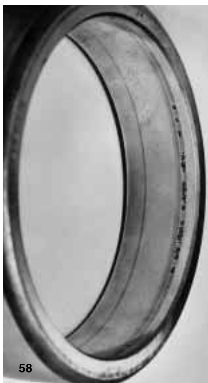
Fig 59 Flaked inner ring of a spherical roller bearing. The extent of the flaking around one entire raceway indicates that the axial load has been very heavy in relation to the radial load
