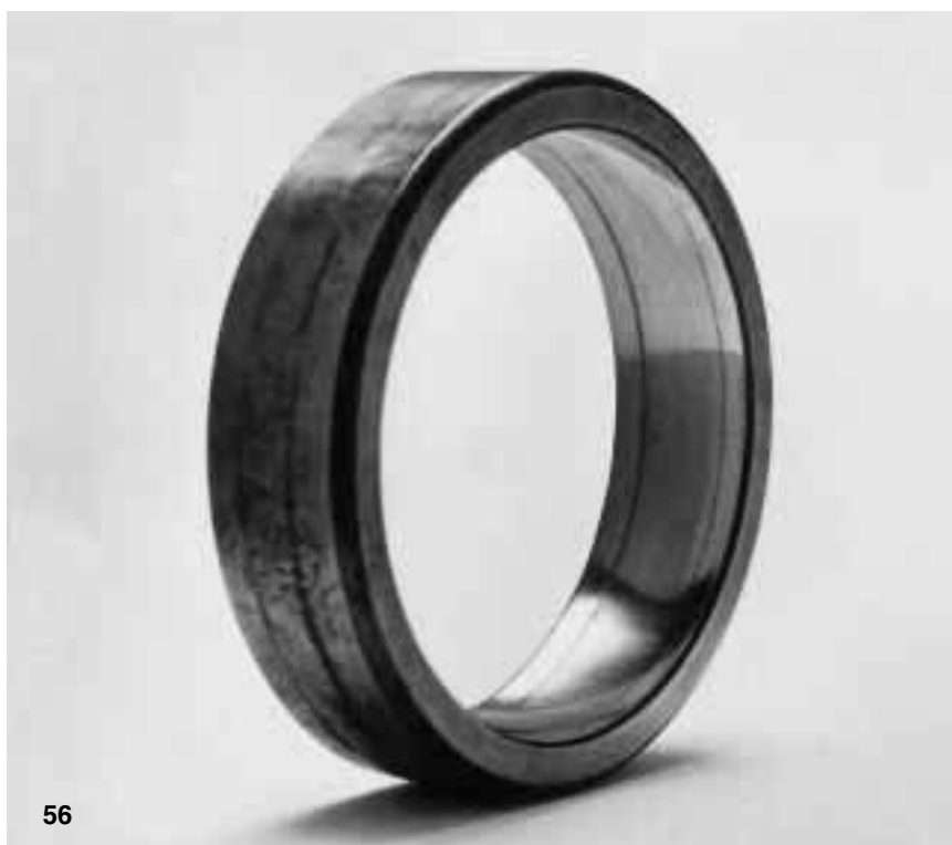
Fig 56 Outer ring of a self-aligning ball bearing that has been driven too far up its tapered seating. The bearing had only performed a few revolutions when the damage was detected. Flaking would soon have occurred if the bearing had been put into service
