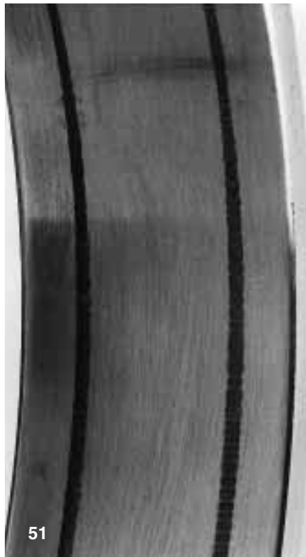
Fig 50 Fluting, caused by the passage of electric current, in the outer ring of a spherical roller bearing
