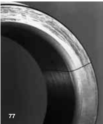
Fig 77 Spherical roller bearing inner ring that has cracked right across following smearing of one face. The ring has been mounted to abut a spacer that has not had a sufficiently tight fit on the shaft. Consequently the spacer has rotated relative to the shaft and the bearing ring
