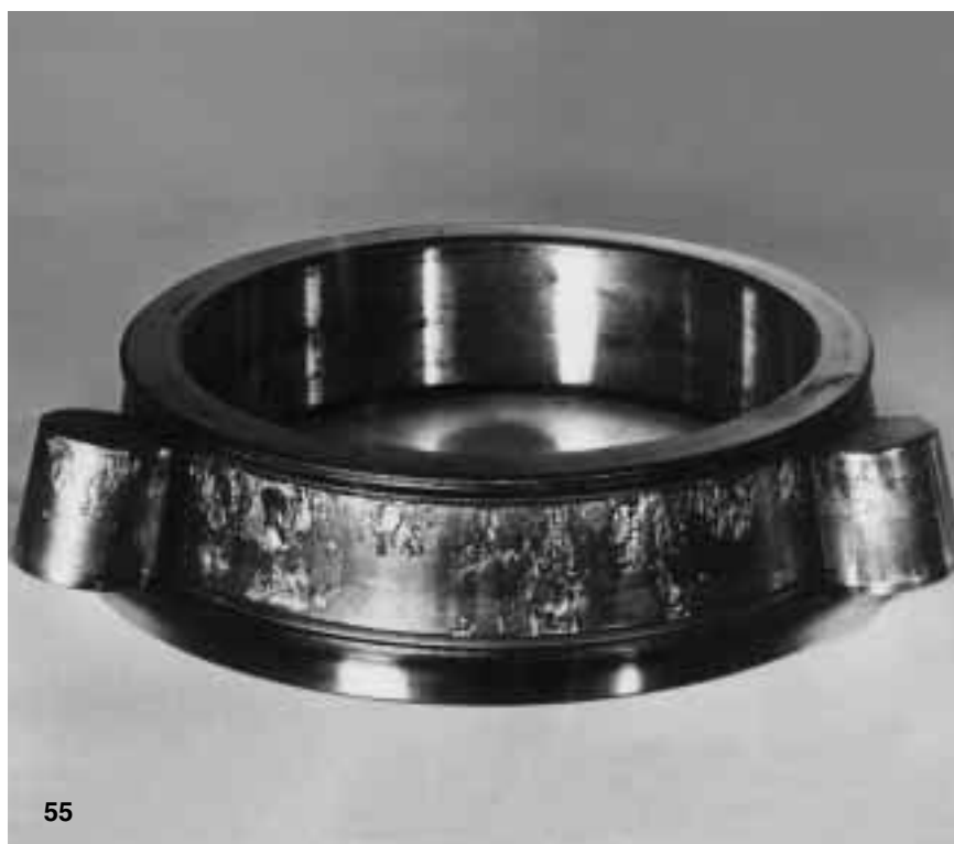
Fig 55 Flaked cone and rollers of taper roller bearing. Heavy loading and inadequate lubrication are the causes of this damage
