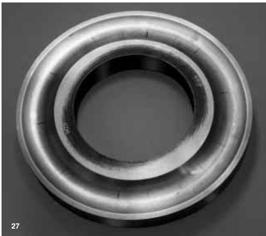
Fig 27 Washer of a thrust ball bearing subjected to overloading while not running. The indentations are narrow and radially aligned, not sphered as in radial ball bearings
