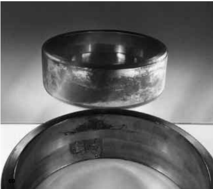
Fig 69 Flaking in the raceways of the outer ring of a spherical roller bearing. Corresponding area of advanced fretting corrosion on the outside surface (for this photograph the ring has been placed in front of a mirror). Development of the corrosion has been accompanied by an increase in volume that has led to deformation of the bearing ring and localised overloading. The results have been premature fatigue and flaking
