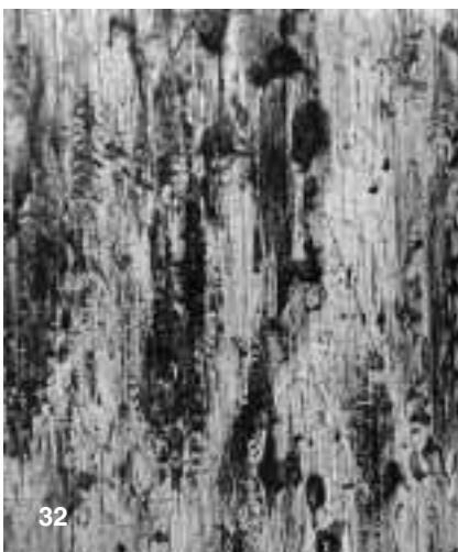
Fig 32 Smearing on the surface of a roller from a spherical roller bearing – 100 × magnification
