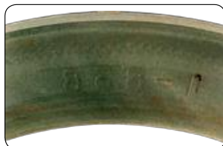
With a polymer spacer: no fretting corrosion after 800 000 km
