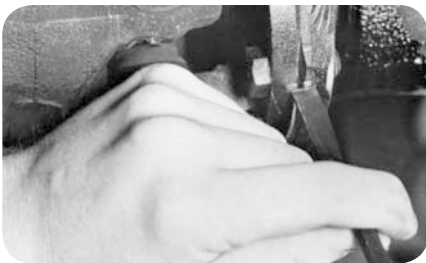
Mark the driveshaft and pinion flange (fig. 39).
