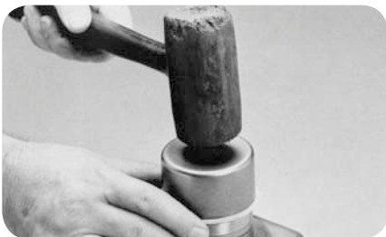
Tap tool to install sleeve over shaft (fig. 47).
