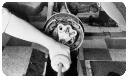
Grip axle shaft flange with a slide hammer (fig. 17).
