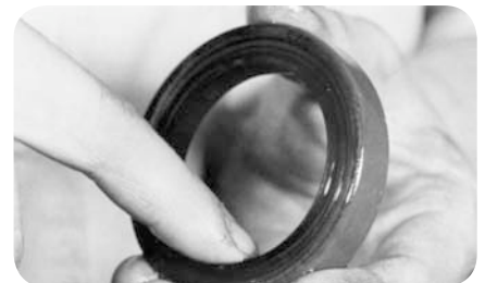
Apply lube to seal lips (fig. 43).
