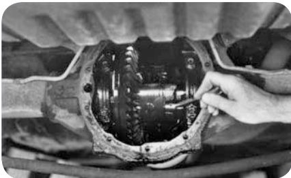
Loosen differential pinion shaft locking bolt (fig. 13).
