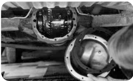
Replace differential cover with new gasket (fig. 21).
