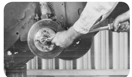
Tighten hub nut while applying brakes (fig. 38).
