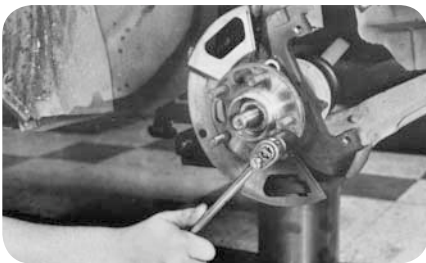
General Motors-Loosen hub/bearing assembly bolts (fig. 27).
