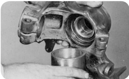
Ford-Place knuckle assembly over spacer tool (fig. 33).
