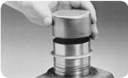
Place Installation tool over Speedi-Sleeve (fig. 46).
