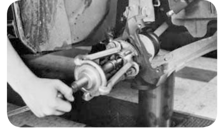
General Motors-Use puller to remove hub bearing assembly (fig. 28)
