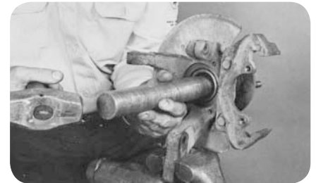
Chrysler-Remove hub from knuckle (fig. 29).
