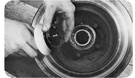
Slide SKF seal onto installation tool (fig. 9).
