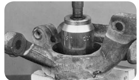
Chrysler-Use socket to press out old bearing (fig. 30).
