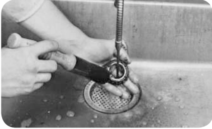
Rinse bearing in clean solvent (fig. 5).
