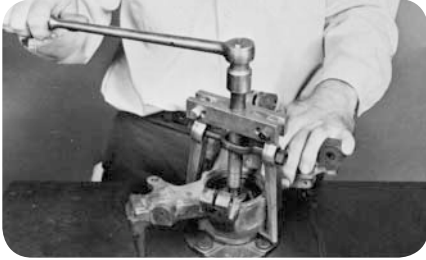
Ford-Grip and remove knuckle from hub (fig. 32).
