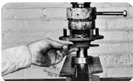
Use arbor press to install bearing (fig. 22).
