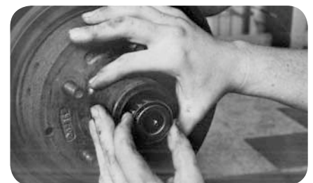
Install outer bearing (fig. 12).
