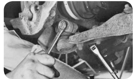
Chrysler-Tighten lower control arm attaching bolt (fig. 36).
