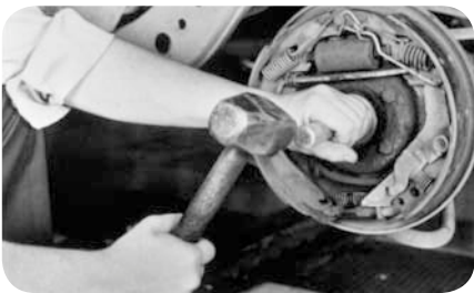
Tap new bearing into shaft cavity (fig. 20).
