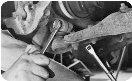
Ford and Chrysler – Loosen bolt on lower control arm (fig. 25).
