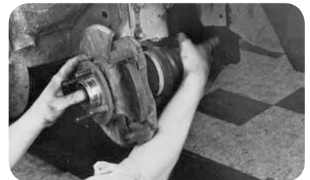
General Motors- Push shaft into hub (fig. 37).
