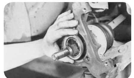
General Motors- Position new seal in bore (fig. 31).
