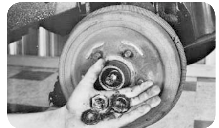
Remove adjusting nut, washer and outer bearing (fig. 3).
