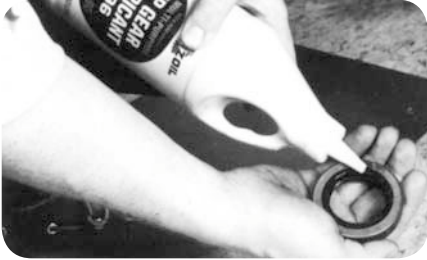
Pre-lube seal with differential lubricant (fig. 19).
