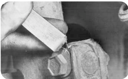
Ford and Chrysler – Mark cam position before disassembly (fig. 26).
