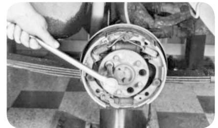
Remove nuts holding retainer plate (fig. 16)
