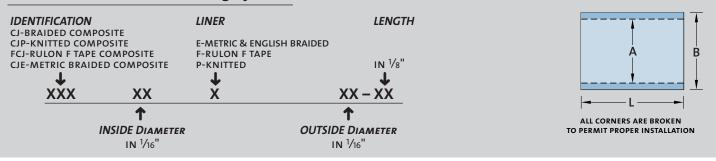
Only braided and RULON D tape lined bearings are available as standard sizes listed in this catalog. Knitted liners and other RULON tapes are available as special orders.
