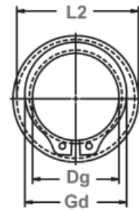
Clearance Diameter & Gaging Diameter Released in Groove.
