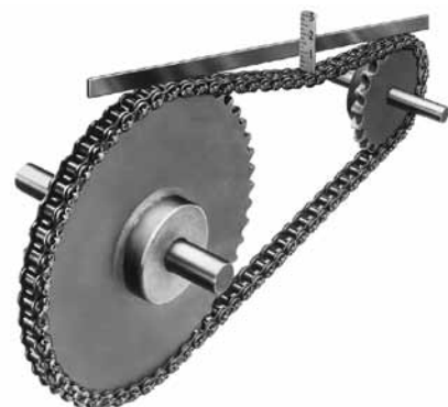
Determining chain sag
