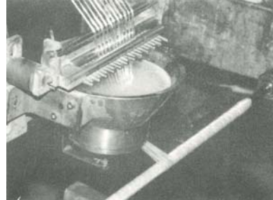
Epoxy coated fiberglass filaments helically wound in overlapping layers.
