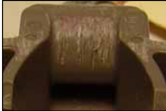
Abrasive sprocket pocket wear
