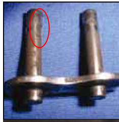
Evidence of overload – deformed pin
