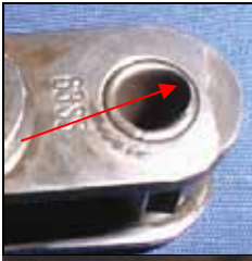
Evidence of overload – deformed bushing
