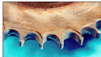
Worn sprocket teeth
