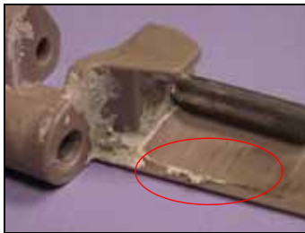
Shavings due to abrasive wear
