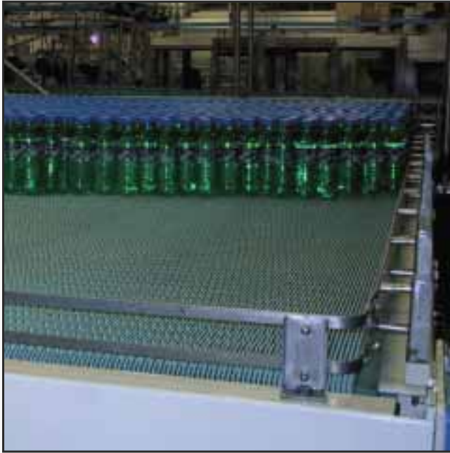
BOTTLE CONVEYOR WITH PLASTIC 2000-SERIES BELT.
