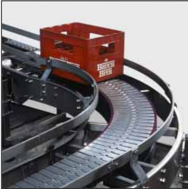
CRATE CONVEYOR WITH SPACE-SAVING MAGNETFLEX® COMBI CURVE.
