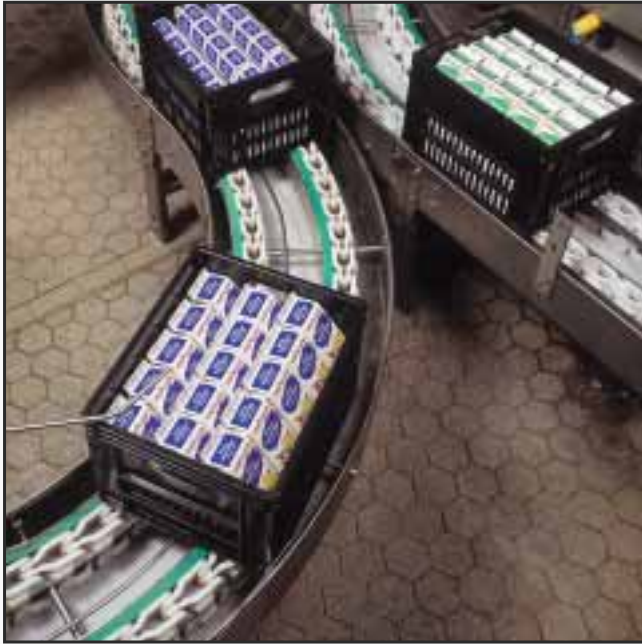
HEAVY DUTY CRATE CONVEYOR WITH PLASTIC CASE CONVEYOR CHAIN.
