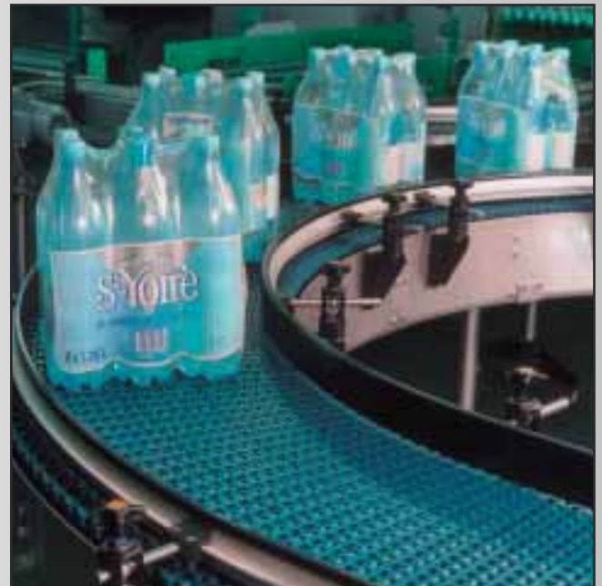
SHRINK-WRAPPED BOTTLES ON 1255-SERIES FLEXBELT.
