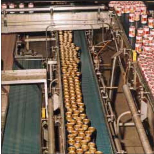
SMOOTH CAN CONVEYORS WITH 500-SERIES PLASTIC BELT.
