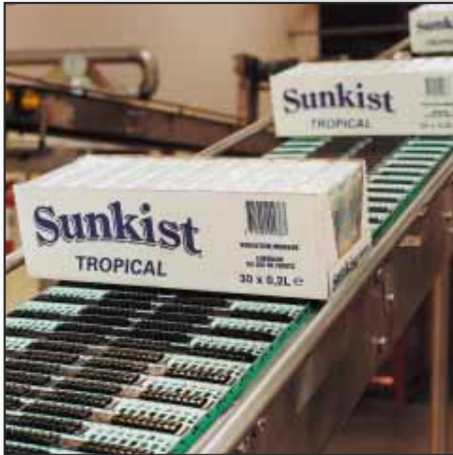
INCLINED TRAY CONVEYOR WITH PLASTIC SUPERGRIP BELT.
