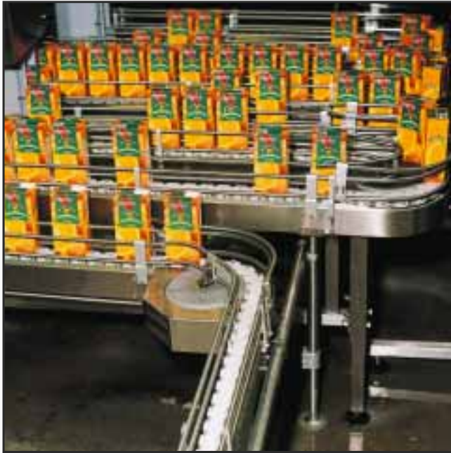
TYPICAL CARTON CONVEYOR WITH PLASTIC MULTIFLEX CHAIN.
