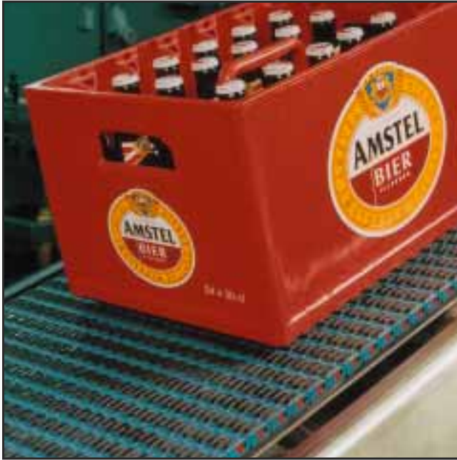
INCLINED CRATE CONVEYOR WITH HEAVY DUTY SUPERGRIP BELT.
