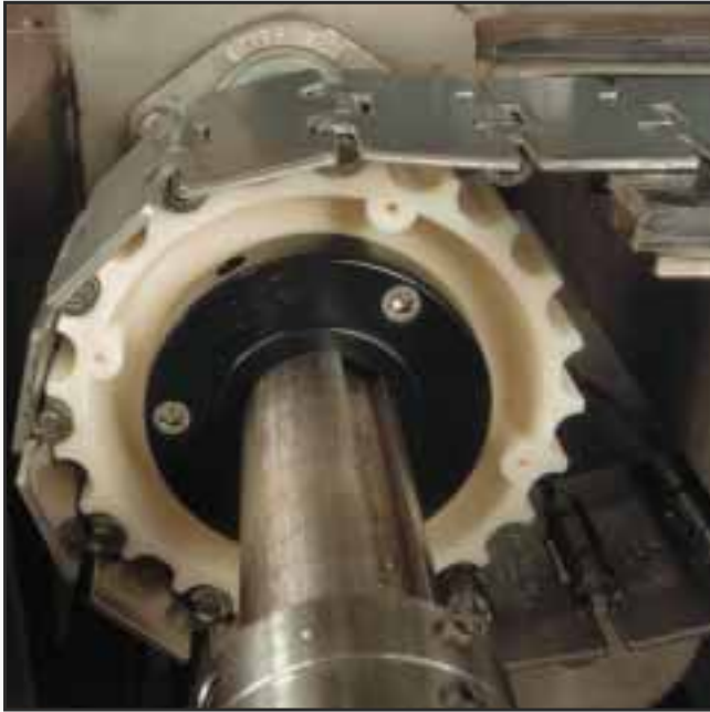
CLASSIC MODU-SPROCKET FOR STEEL SINGLE HINGE AND MAGNETFLEX® CHAINS.
