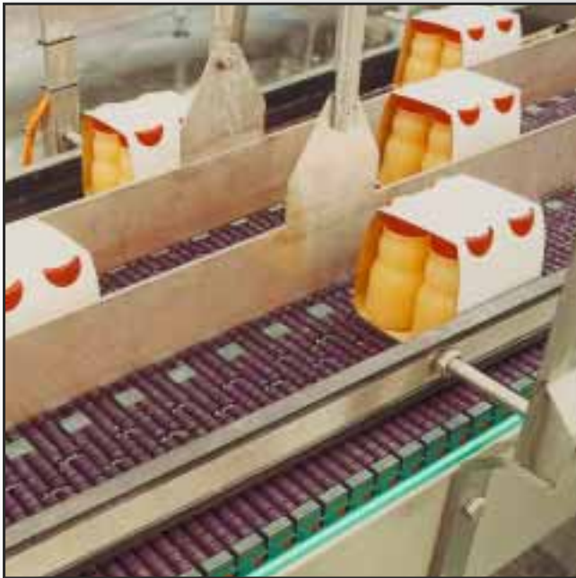
SMOOTH 4-PACKS CONVEYOR WITH PLASTIC 1005-SERIES LBP BELT.
