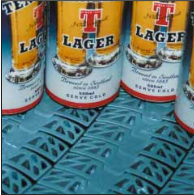
SIDEFLEXING CAN CONVEYOR WITH PLASTIC MAGNETFLEX® 1050 CHAINBELT.
