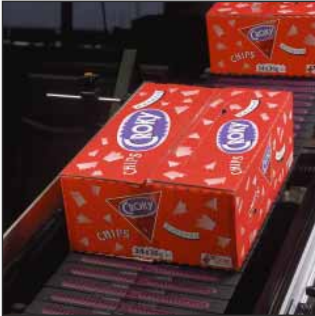
INCLINED BOX CONVEYOR WITH PLASTIC SUPERGRIP CHAIN.
