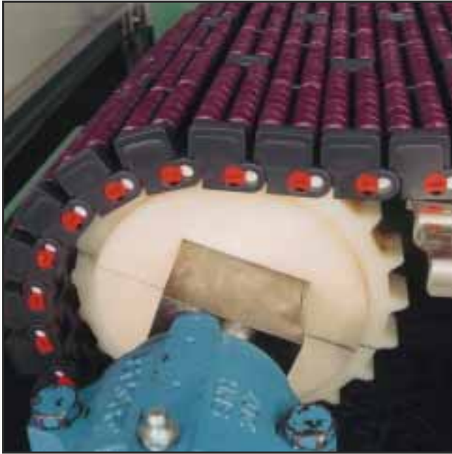
CONVEYOR WITH TIME-SAVING PLASTIC SPLIT SPROCKETS.
