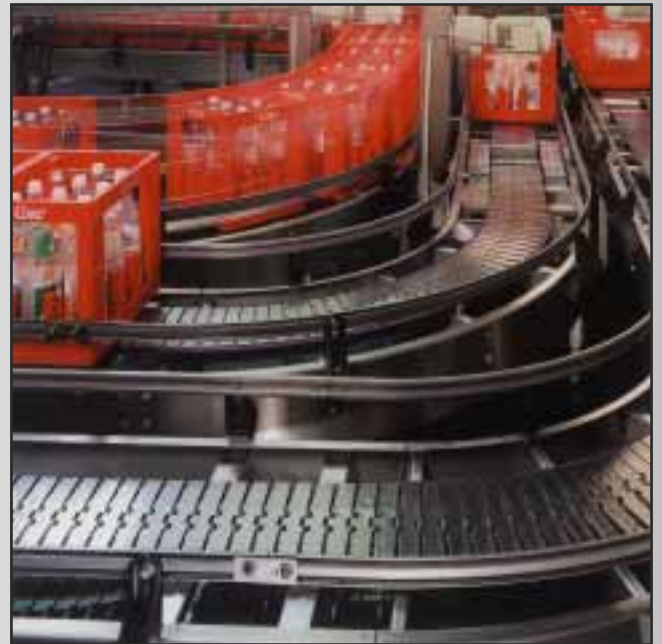
CASES ON WEAR-RESISTANT 60-SERIES MAGNETFLEX® CHAIN.
