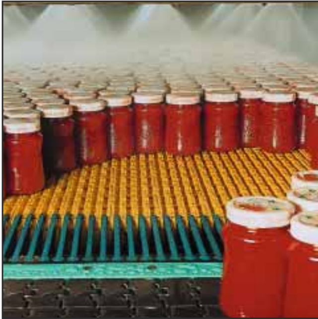
HEAVILY LOADED GLASS PASTEURIZER OUTFEED WITH PLASTIC 2500-SERIES BELT.
