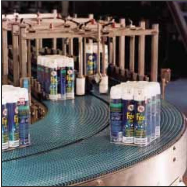
SIDEFLEXING AEROSOL CAN CONVEYOR WITH 505-SERIES PLASTIC FLEXBELT.
