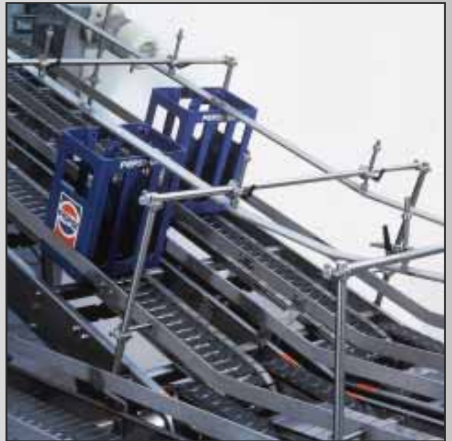
CRATES ON INCLINING DOUBLE HINGE CHAIN WITH RUBBER TOP.
