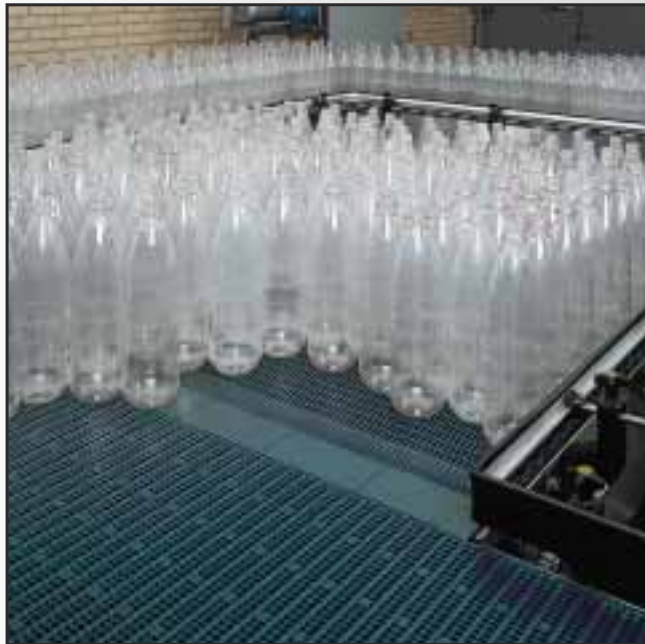
SMOOTH BOTTLE TRANSFER WITH PLASTIC CLICK-COMB FINGERPLATES.
