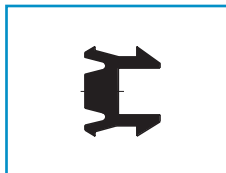
Part. 370 - Pag. S70 Sealing profile for Part.422. Improves Guide cleanliness.
