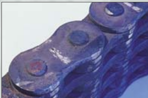
Loose link pins.
