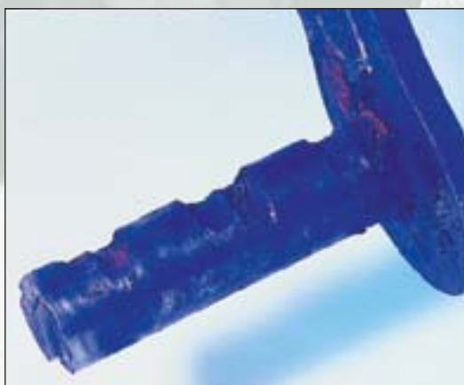
Wear on the chain pin.
