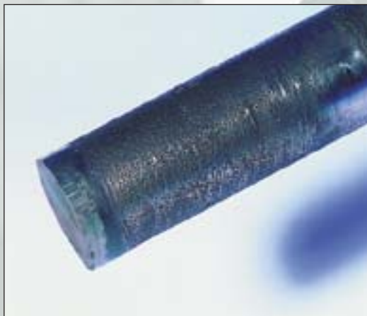
Pitting on pin and plate.
