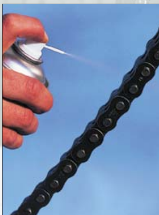
Lubricating with spray can.
