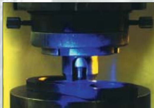
Link plate during Rockwell hardness measurement.
