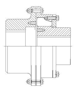
Coupling with long boss inner member and large boss driving flange for use on vertical applications.
