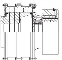
Combination with a torque limiting device to prevent damage to driving and driven machine under shock load.
