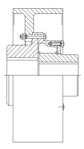
Coupling with brake drum for use on cranes, fans and conveyor drives, (brake disk couplings are available).
