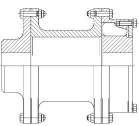
Spacer Coupling. Used to increase distance between shaft ends and allow easy access to driven and driving machines.
