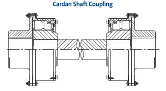
Cardan Shaft Coupling. Used to increase the distance between shaft ends and give a higher misalignment capability.
