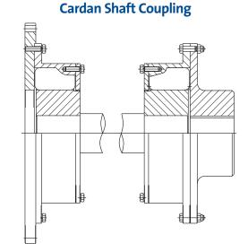
Cardan Shaft Coupling. Used to increase the distance between shaft ends and give a higher misalignment capability.
