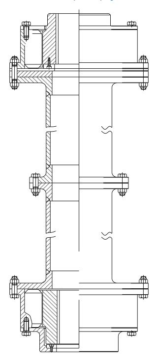
Spacer Couplings. Used to increase the distance between shaft ends and allow access to driven and driving machine.
