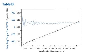
Table D shows the equivalent Renold Hi-Tec Couplings engineered solution using a PM coupling.
