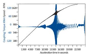
Table A shows vibrating torque experienced in the motor shaft when the system is connected rigidly (or by a gear or membrane coupling) to the driven system.
