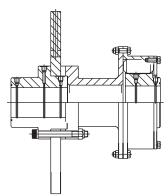
Combination with a brake disc, for use on cranes, fans and conveyor drives. (Brake drum couplings also available).
