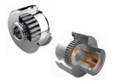
**SA** Suitable for all small machine applications due to compact design Grease lubricated, sealed for life with hardened chromised steel sprags as standard
