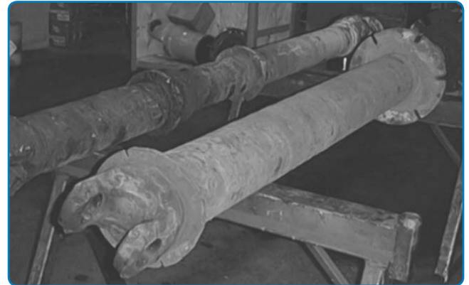
A universal joint, as received from a customer, at our service center for inspection and rebuilding
