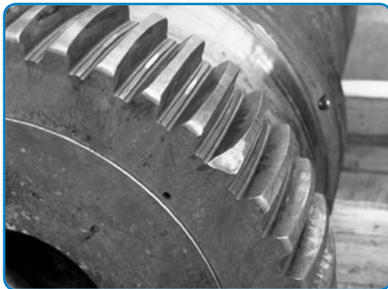
Tooth End Breakage due to over-misalignment
