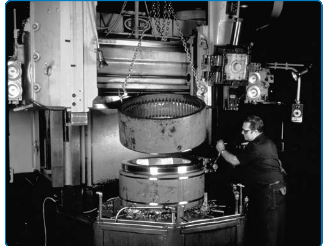
A damaged gear ring is machined off a spindle roll sleeve; The cost to repair is typically about half the cost of replacement
