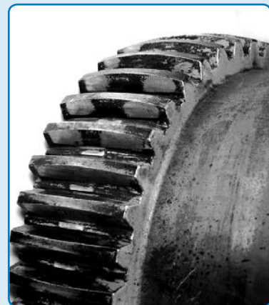
Lapped Gearing with blue contact check at 3° 60-70% gear teeth in contact Good finish, corrected for carburizing distortion
