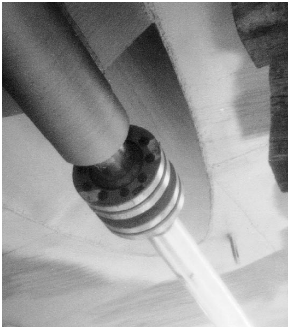
Fig. 32 · Supply ship The propeller-shafts are connected with Shrink Discs 240 RfN 4091. Messrs. Mangone Shipbuilding, USA
