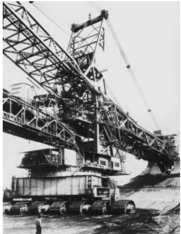
Fig. 26 · Bucket wheel excavator. Locking Assemblies RfN 7012 used in bucket wheel, the bucket wheel drive, travelling gear drive, the belt drums, etc. Messrs. Krupp, works photograph
