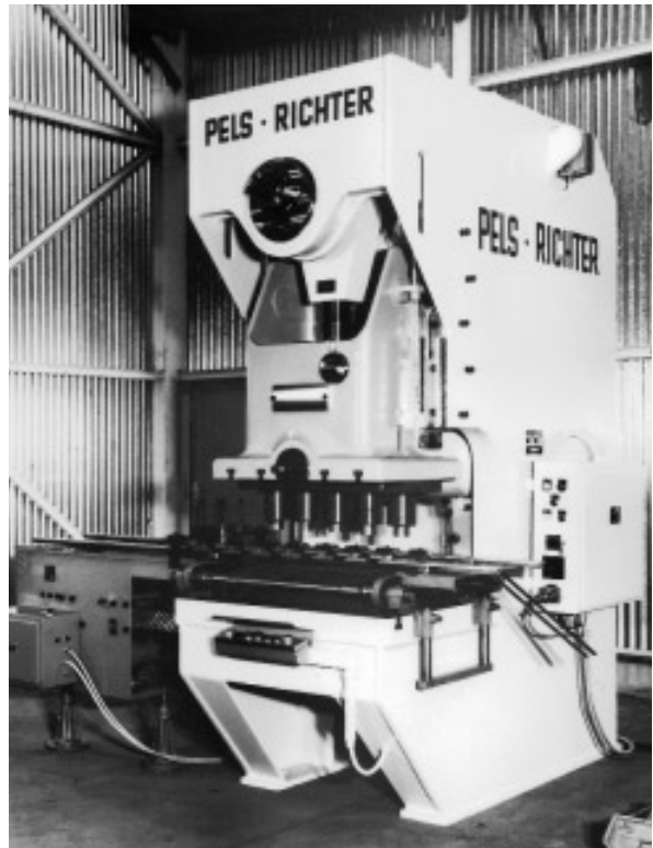
Fig. 30 · Single-column eccentric press. Gearwheels mounted on the crankshaft with Locking Assemblies RfN 7012. Messrs. A. Richter, Kassel-Lohfelden, works photograph
