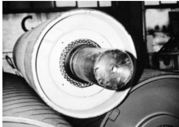
Fig. 36 - Conveying belt drums. Mounted on the drum shaft using Locking Assemblies RfN 7012. Messrs. Italsider Co./Italy
