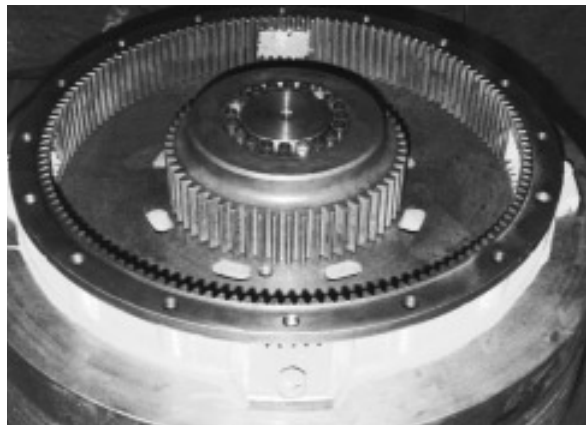
Fig. 44 - Bolt forming machine. Pinion mounted with Locking Assembly 120 x 165 RfN 7012. Messrs. Sakamura Machine Mfg. Co. Ltd., Japan
