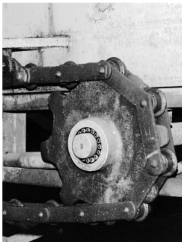
Fig. 46 - Chain conveyor. Sprockets mounted with Locking Assemblies 70 x 110 RfN 7012. Messrs. Hitachi Zosen Co. Ltd., Japan
