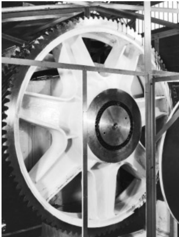
Fig. 25 · Crank press. Gearwheel mounted with Locking Assemblies RfN 7012. Messrs. Hatebur, works photograph
