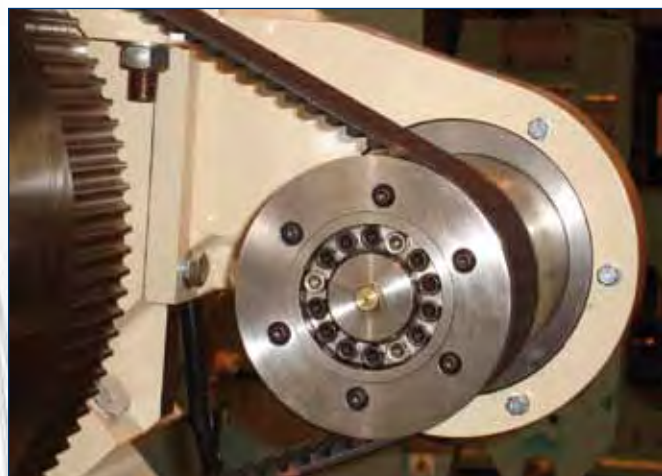
Locking Assembly RfN 7012/RfN 7012-IN · Belt pulley
