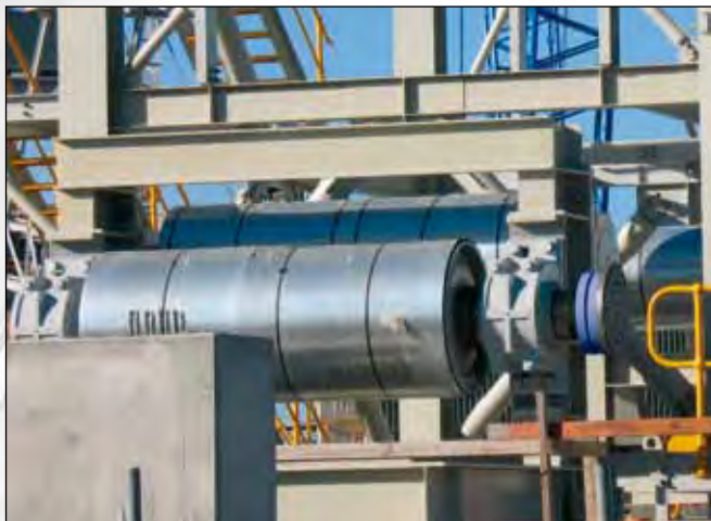
Conveyor Pulley with Locking Assemblies and a Shrink Disc® on the drive side
