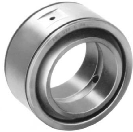
A spherical plain bearing with O-ring grooves to seal the O.D. against the housing and special lubrication holes in the O.D. of the outer ring. This bearing is used in the upper position of the articulating joint of a front end loader.
