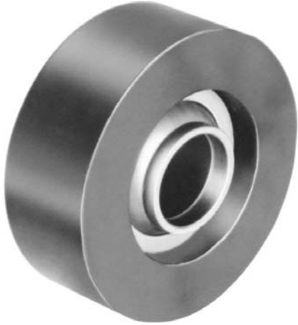
A thin dense chrome coated extended inner ring spherical plain bearing is pressed into a roller and used in a flexible conveyor train in underground coal mines. The thin dense chrome is used for its corrosion resistance properties.
