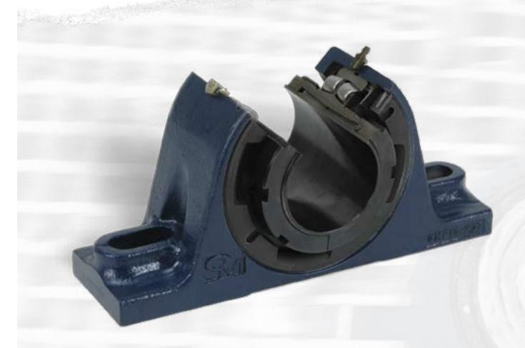
The patented double-taper design of V-Lock™ bearings makes installation and removal a snap. You no longer have to set clearances or remove stubborn bearings. And, the unique locking mechanism virtually eliminates fretting corrosion.
