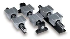
PowerTrax<sup>™</sup> Series 100 slide systems are pre-assembled and ready to mount. Series 100 slides consist of combinations of PowerTrax<sup>™</sup> Linear Ball Bearing Pillow Blocks, HG shafting, carriage plates and shaft supports. Aluminum carriage plates include threaded steel inserts at key mounting locations. All exposed non-wearing components have a protective, corrosion resistant finish.
