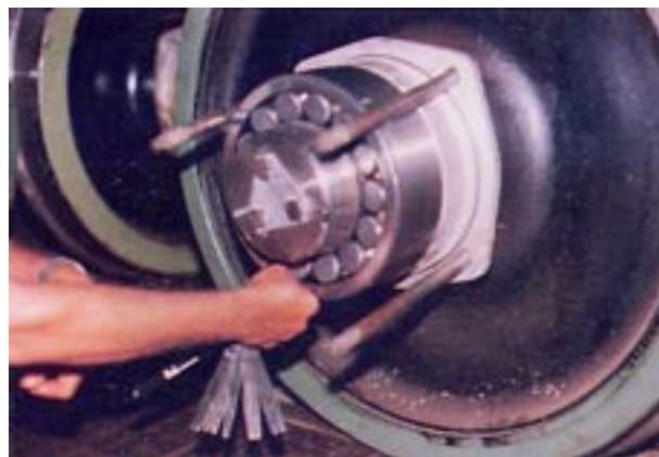
Fig 19 Checking Brg. radial clearance in mounted condition
