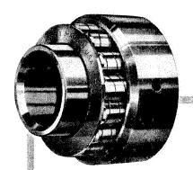
High capacity cylindrical roller bearings made in three dimensional series, wide and narrow widths, to standard AFBMA dimensions. There are ten major types—for radial loads, or light or intermittent thrust loads. Of the ten types, two have non-separable component parts, four have separable inner races, four have separable outer races, thus permitting flexibility in machine design and assembly procedures. Separable race can
