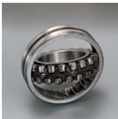
Open-type bearing after testing (change in grease color due to contamination with breeze)
