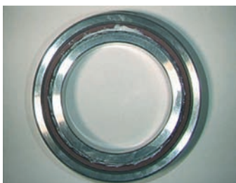
Photo. 6.1 Filling grease into angular contact ball bearing
