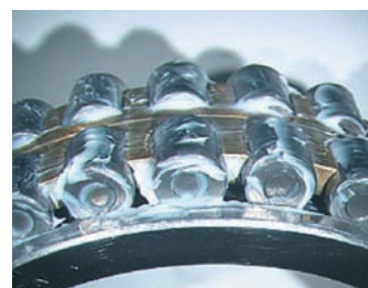
Photo. 6.2 Filling grease into cylindrical roller bearing
