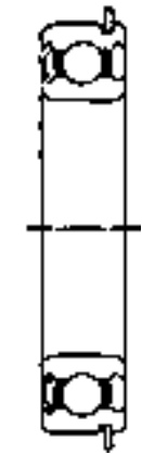
Single Shielded With Snap Ring 62ZNR
