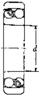
Tapered Bore 12K Taper 1:12
